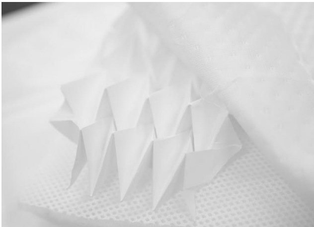
Figure 3. Ticking folded open, showing the origami layer folded up.
