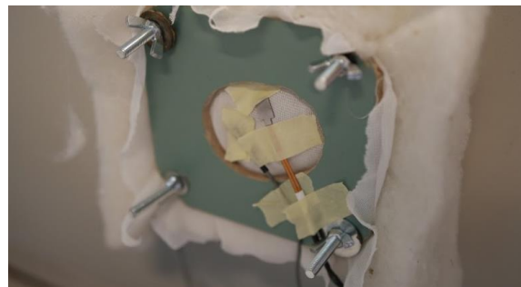
Figure 6. The brace that hold the testable material. Sensors are attached as well.
