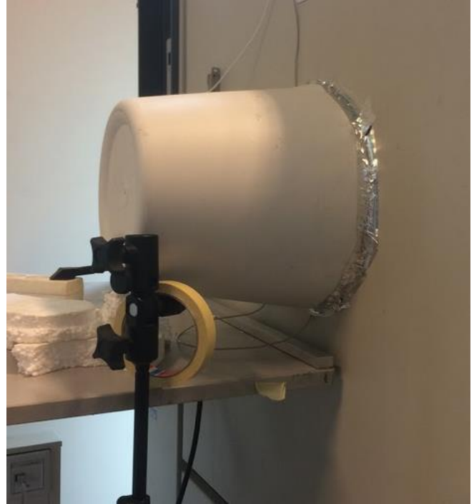
Figure 4. The insulating hood attached to the climate chamber.
