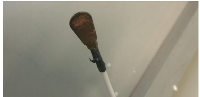
Figure 5. One of the used temperature sensors
